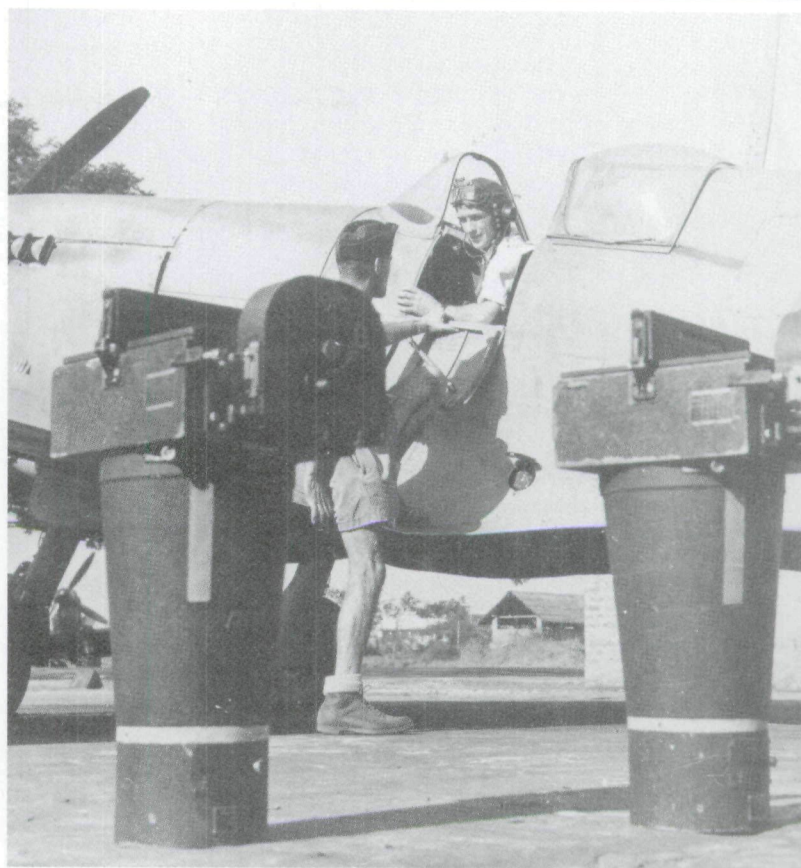
A photo reconnaissance Spitfire with two F-52 cameras in the foreground. The cameras were located in the fuselage of the aircraft and the long 40 inch lenses enabled pilots to photograph objects from a height of about 30,000 feet. Each 8½ by 7 inch photo covered an area of about a square mile with sufficient detail to identify a vehicle on the ground.
